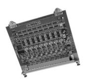
The Model 7003-8-LVDT is used in conjunction with the Model 7003-8-A-I Analog Input Card to perform signal conditioning, polarity demodulation and AC excitation for transformer type transducers.
