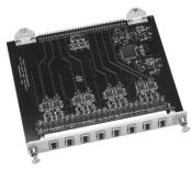
The Model 7003-8-TC Thermocouple Input Card is used in conjunction with the Model 7003-8-A-I Analog Input Card to perform signal conditioning and cold-junction compensation for thermocouple types J, K, T, E, N, R, S, and B.
