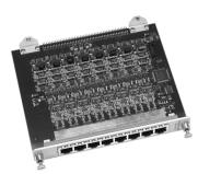
A choice of two Strain Gage Input Cards (7003-8-SG or 7003-8-SG-A) are used in conjunction with the Model 7003-8-A-I Analog Input Card to perform bridge excitation, bridge completion, shunt calibration, and signal conditioning for eight quarter, half, and full bridges. Note that the 7003-8-SG-A Strain Gage Input Card with Analog Output has an analog output which provides an amplified representation of the input source.
